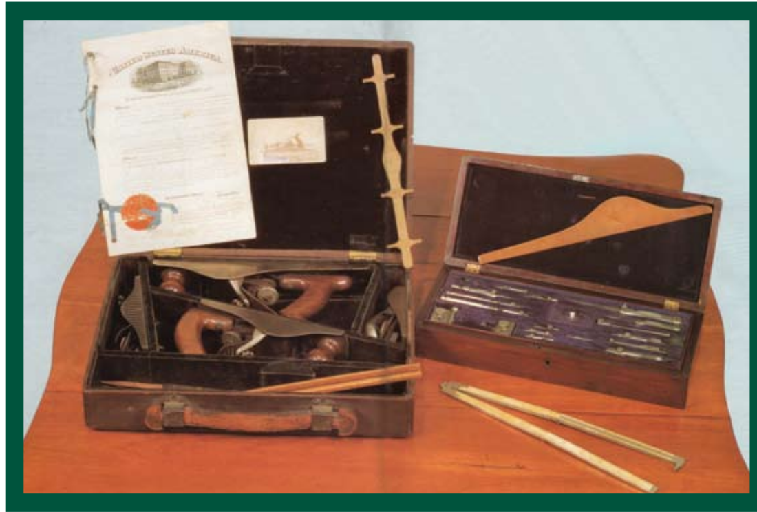
ABOVE: Louis Rodier's personal traveling display case with two bench planes and two block planes that were prototype models for his April 21, 1885 Patent. Also shown is Rodier's drafting set patterns, vintage photograph of his plane and the original patent certificate for his 1885 patent.
