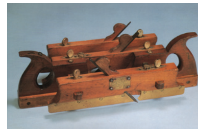
Jones Shoot Board Plane: Possibly the patent model, patented by Joseph Jones. Brass name plate stamped "Jones Patent Feb 20, 1866".
