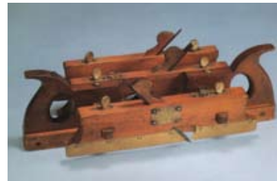
Jones Shoot Board Plane: Possibly the patent model, patented by Joseph Jones. Brass name plate stamped "Jones Patent Feb 20, 1866".
